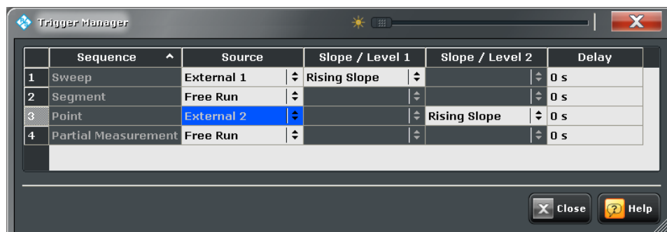
Fig. 4-29: Example of a multiple trigger configuration
