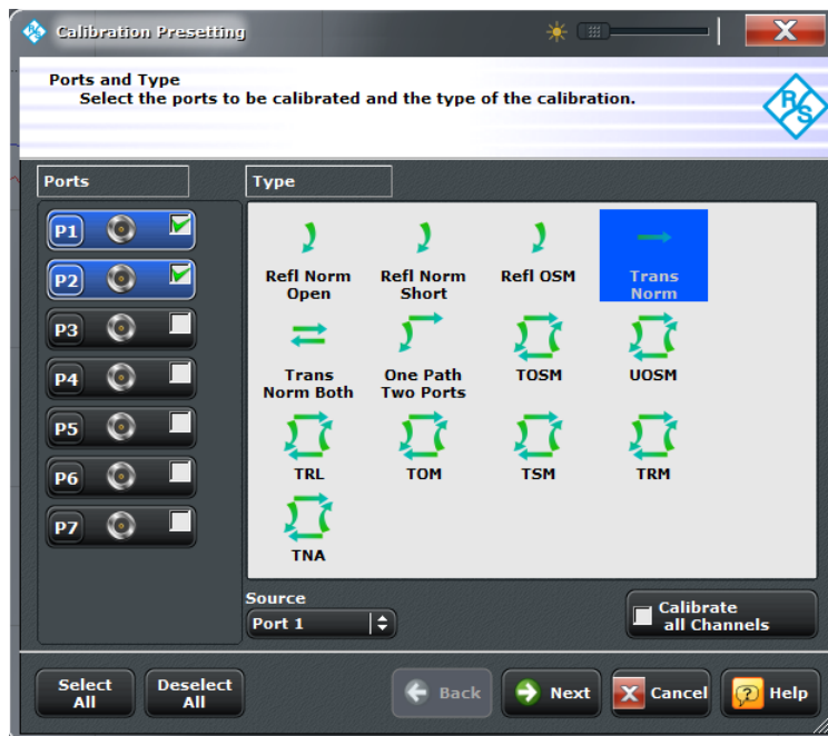
Fig. 4-10: Calibration Presetting: Ports and Type (> 4 test ports)
