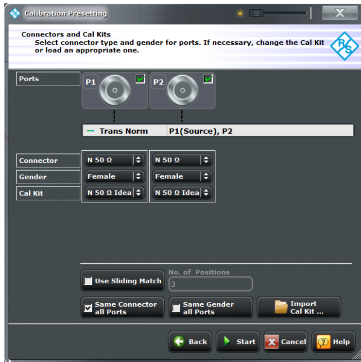
Fig. 4-11: Calibration Presetting: Connectors and Cal Kits
